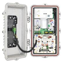
The node can also be populated with other single-slot ARRIS node modules such as an optical switch or EDFA, optimizing performance and reliability for a wide roange of applications. When deployed the Remote Phy module occupies all three available slots, generating the forward signals and providing the return path connectivity for the node.
